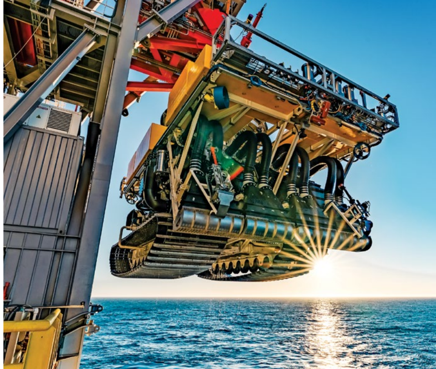
A nodule collection vehicle is ready to be launched from a mining ship.
